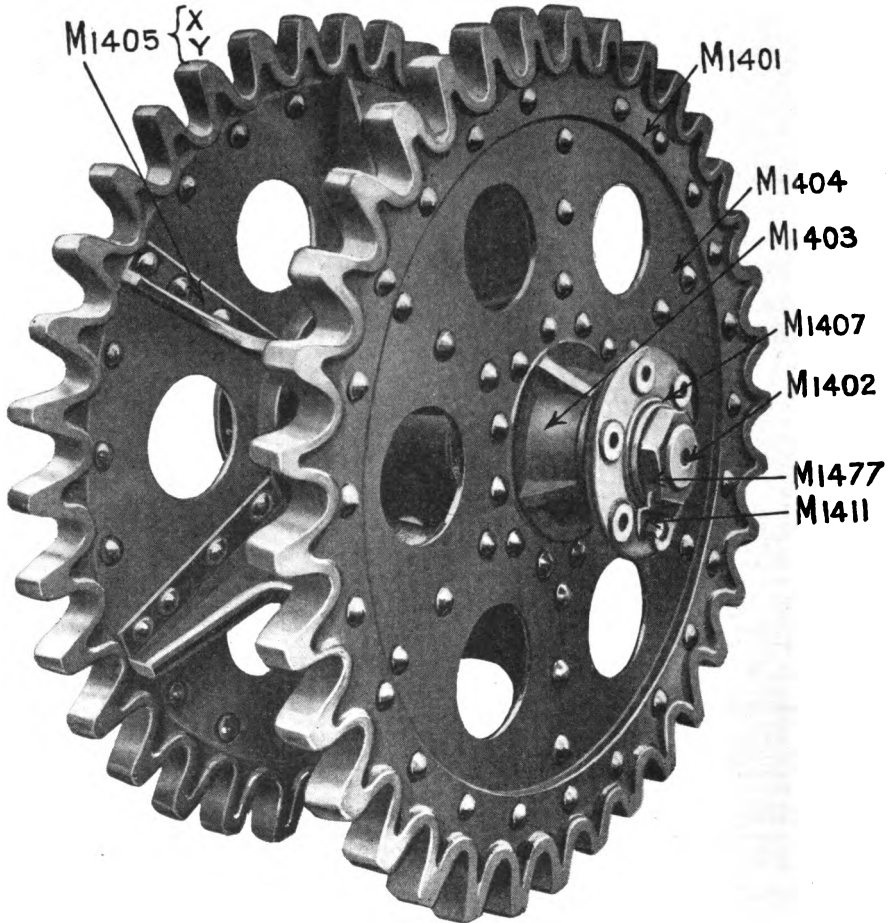
ROAD TRACK DRIVING WHEEL
